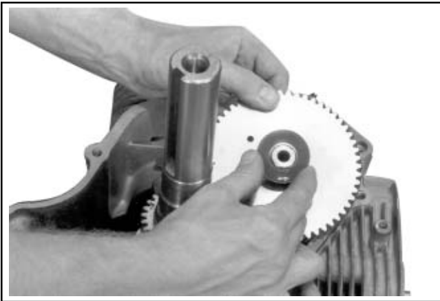
Figure 11-15. Change Shim to Obtain Correct End Play.
